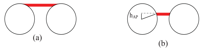
Fig. 8. Variation of the mobile layer span (width) within the boundaries of the large AP particles during regression: a) maximum span (left); b) smaller span (right).
