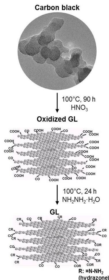
Fig. 1. Sketch of the two-step method for the preparation of GL layers from CB.
