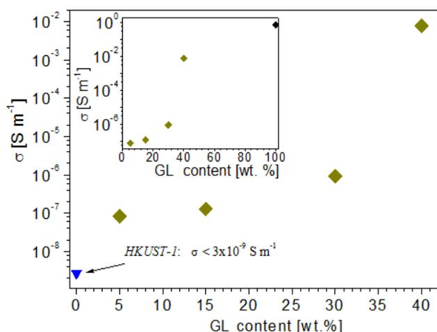
Fig. 5. (color online) electrical conductivity of HKUST-1 (blue), MGL composites (green), and GL (black). (adapted from [70]).
