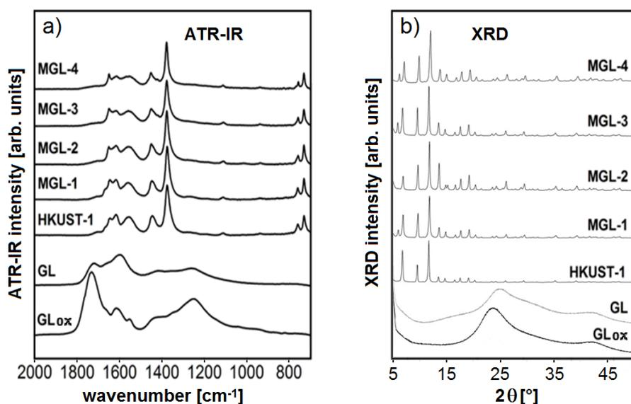
Fig. 4. a) ATR-IR spectra and b) XRD patterns on parent compounds and MGL composites. (adapted from [70]).
