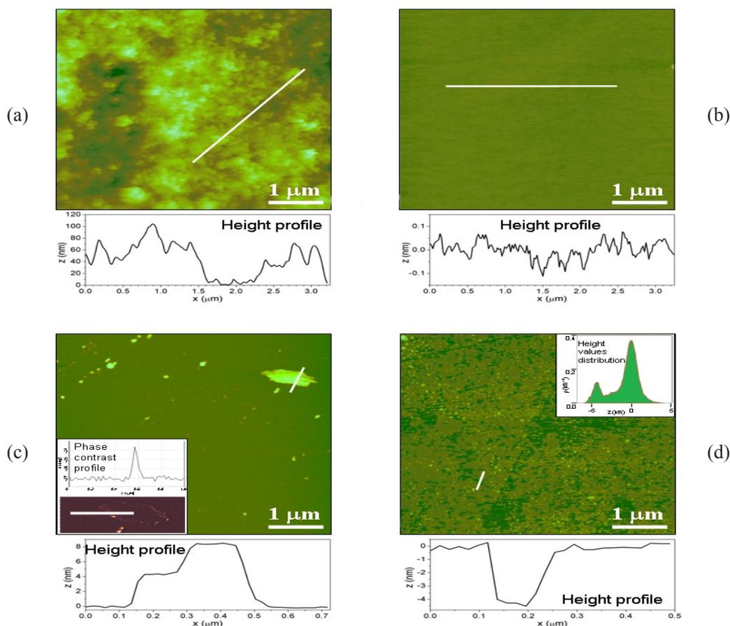
Fig. 3.  $5\ \mu\text{m} \times 5\ \mu\text{m}$  AFM images on the four investigated GL samples, together with line profiles: a) Sample A; b) Sample B; c) Sample C (in the inset, the phase contrast profile on a line crossing the large “island” on the top-right of the image); d) Sample D (in the inset: histogram of the distribution of measured height values on the image). (adapted from [66]).
