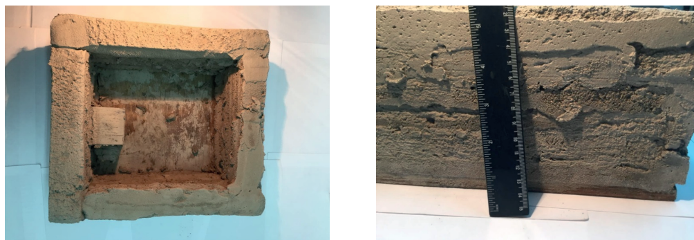
Fig. 12. The square of cement walls, printed on the pilot setup.
