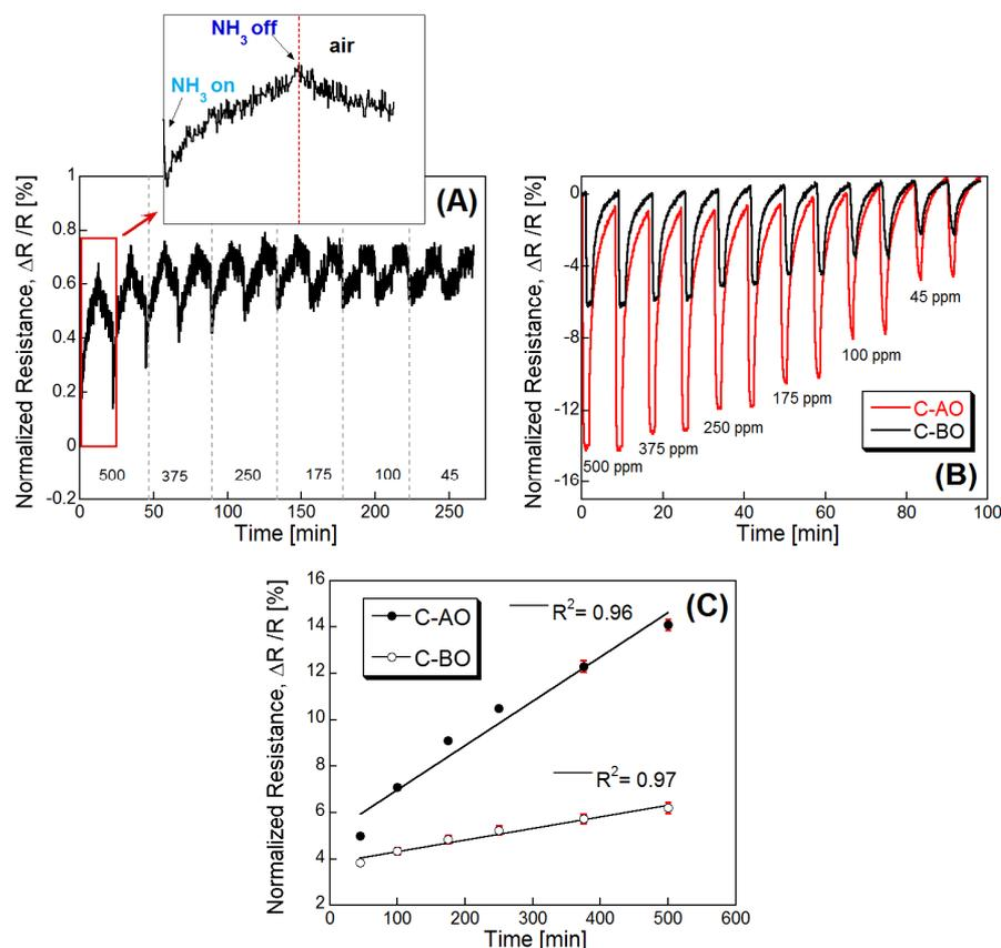
Fig. 4. Response curves for C-B (A), C-AO and C-BO (B) exposed to various ammonia concentrations. (C) Dependence of  $\Delta R/R_0$  of the oxidized samples on  $\text{NH}_3$  concentration. The error bars are similar or smaller than the size of the data points used. Reprinted with permission from Ref. [24]. Copyright 2016, Elsevier.
