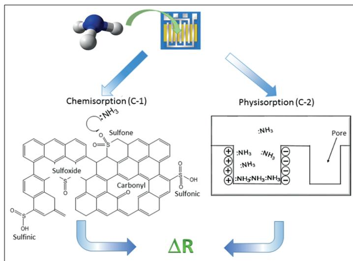
Fig. 5. Visualization of the working principles of the nanoporous-carbon based sensor (only sulfur-containing groups active in adsorption of  $\text{NH}_3$  are presented on the surface of the C1-carbon). Reprinted with permission from Ref. [23]. Copyright 2015, Elsevier.
