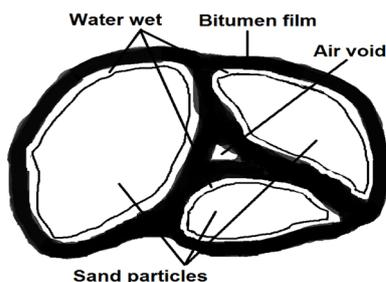
Fig. 7. Composition and structure of oil sands.
