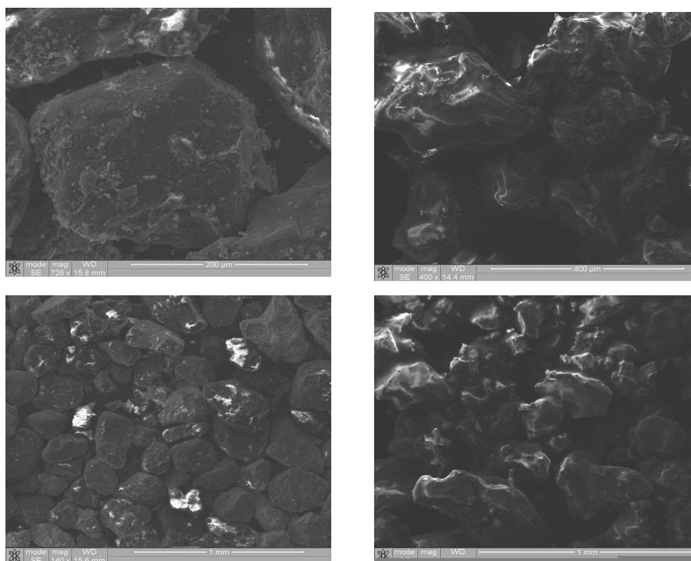
Fig. 5. SEM image of oil sand and after thermal extracted sand.
