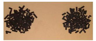
Fig. 1. A photo of the granulated samples of the catalyst containing FMNs: Fe-Mn(Al) on the left and Fe-MN(Ca-M) on the right.
