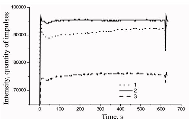
Fig. 3. Concentration profiles of distribution of the oxides-components of the ferrite over the  $\text{NiFe}_2\text{O}_4$  film depth: 1 –  $\text{Fe}_2\text{O}_3$ ; 2 –  $\text{FeO}$ ; 3 –  $\text{NiO}$ .
