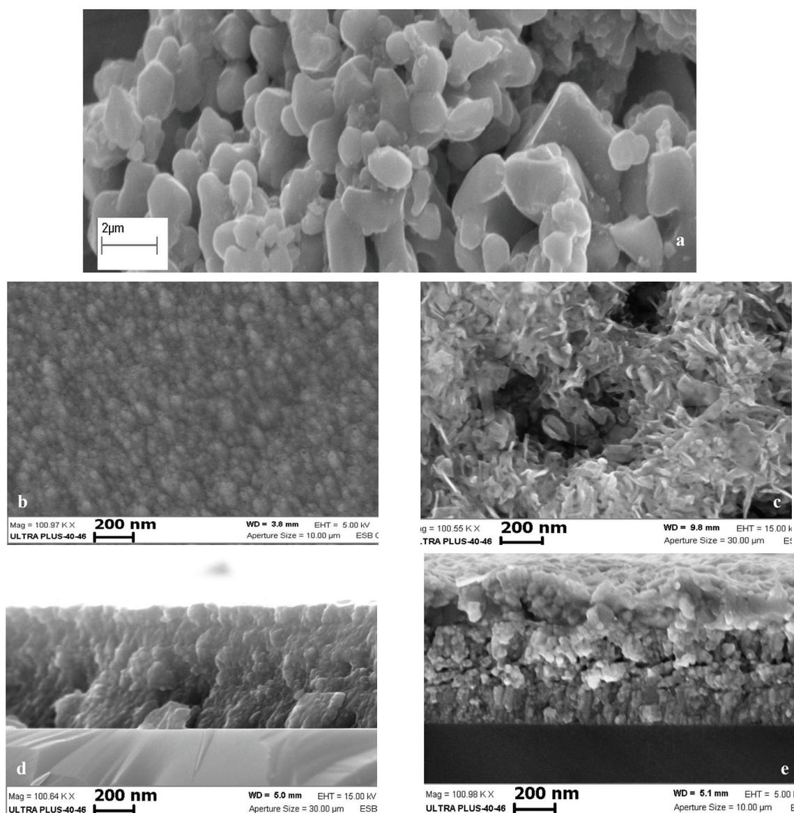
Fig. 1. Microstructure of the green powder (a) and a thin film of  $\text{NiFe}_2\text{O}_4$  ferrite on the support Si (100) after ion-beam sputtering (b – surface, d – transverse fracture) and after annealing at 770 K/90 min in the air (c – surface, e – transverse fracture).
