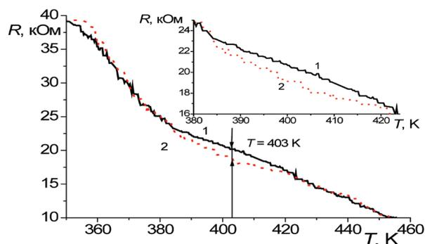
Fig. 2. The temperature dependence of the electrical resistance of the NiFe<sub>2</sub>O<sub>4</sub> thin film deposited on the Si (100) support.
