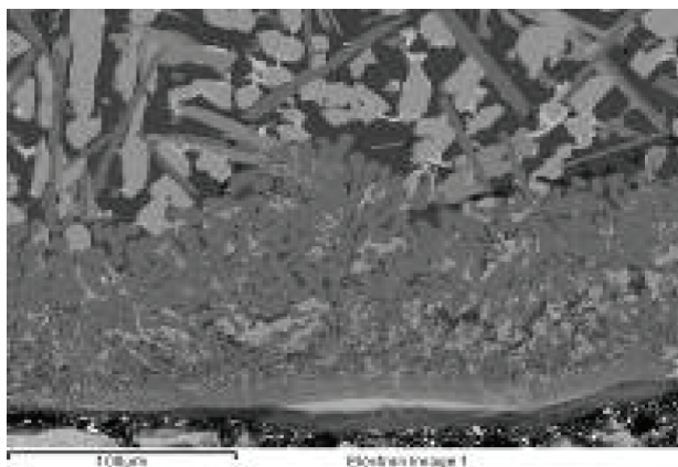
Fig. 15. The microstructure of an upper layer of the SHS product synthesized under microgravity.
