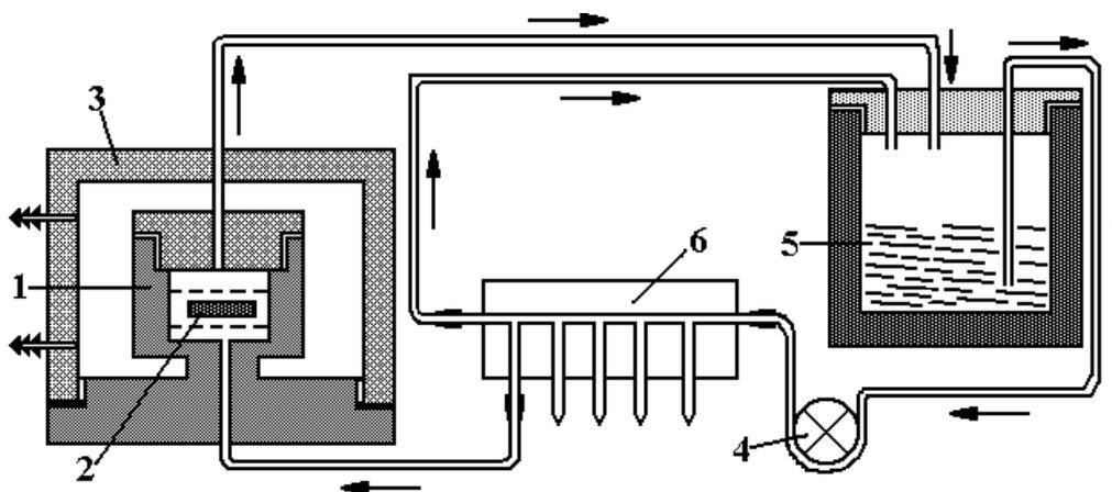
Fig. 2. Installation for the study of the release kinetics of drugs immobilized on polymeric supports. 1 – sample cell; 2 – tablet made of the product under study; 3 – thermostated cell; 4 – peristaltic pump; 5 – eluent reservoir; 6 – flow regulator.
