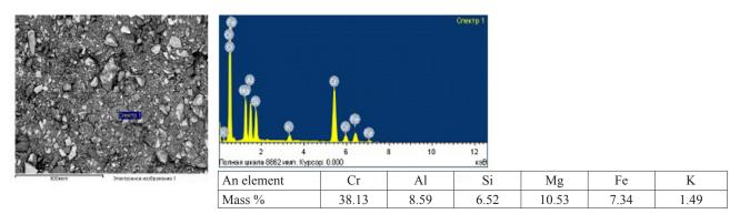
Fig. 11. The elemental composition of the calcined chromite pellets containing 15 % of the internal overburden rock and 2% of coal fines (spectrum 1).
