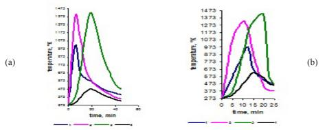
Fig. 4. Temperature: 1 - in the furnace; 2 - at the depth of 100 mm from the surface of the pellets; 3 - at the depth of 200 mm; 4 - on the roasting grate (400 mm from the surface of pellets).
