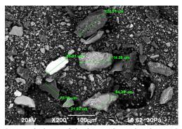
Fig. 6. Morphology of the internal overburden rocks on a reflected electron probe (x200).
