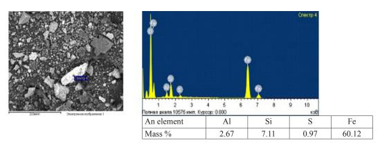
Fig. 9. An elemental composition of the internal overburden rock a) spectrum 1; b) spectrum 2; c) spectrum 3; d) spectrum 4.
