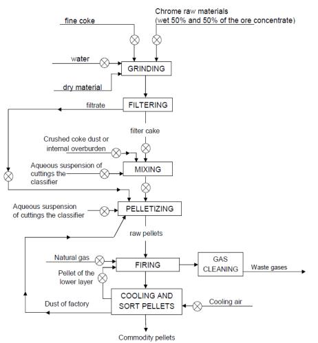
Fig. 1. A schematic diagram of pellets manufacture.
