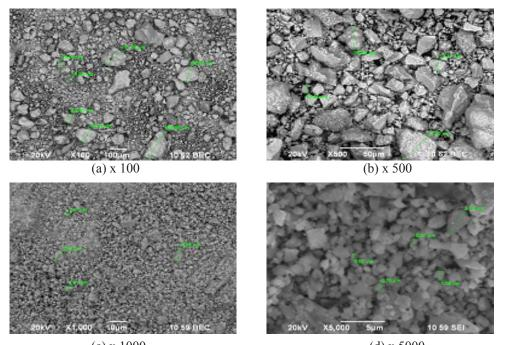
(c) x 1000 (d) x 5000 Fig. 7. Morphology of the off-grade chromite ores on a reflected electron probe.
