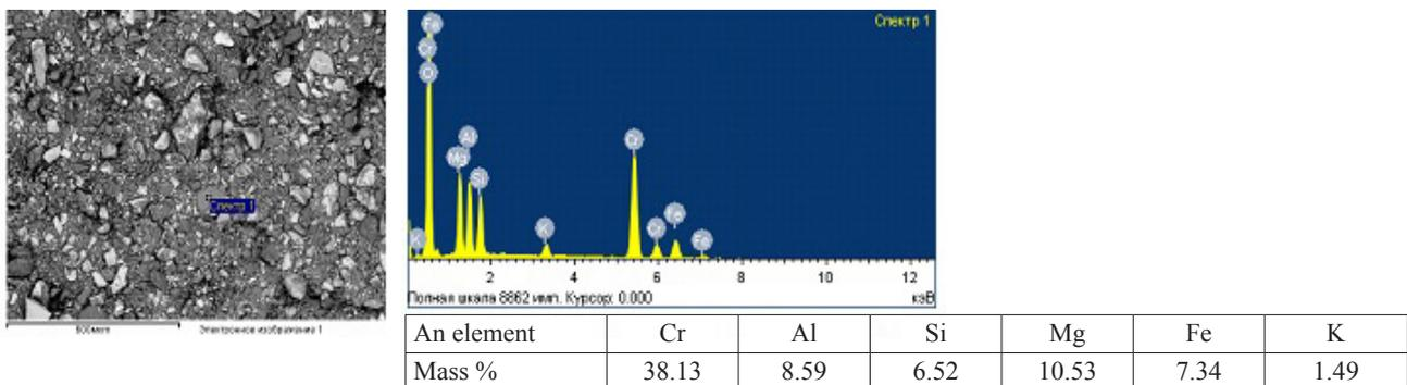
Fig. 11. The elemental composition of the calcined chromite pellets containing 15 % of the internal overburden rock and 2% of coal fines (spectrum 1).
