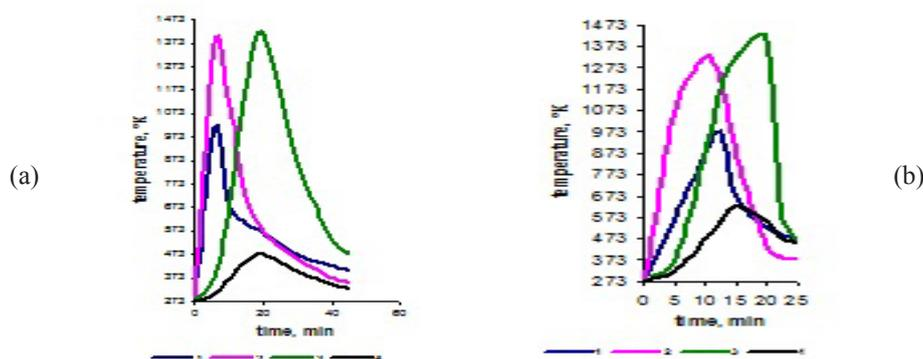
Fig. 4. Temperature: 1 – in the furnace; 2 – at the depth of 100 mm from the surface of the pellets; 3 – at the depth of 200 mm; 4 – on the roasting grate (400 mm from the surface of pellets).
