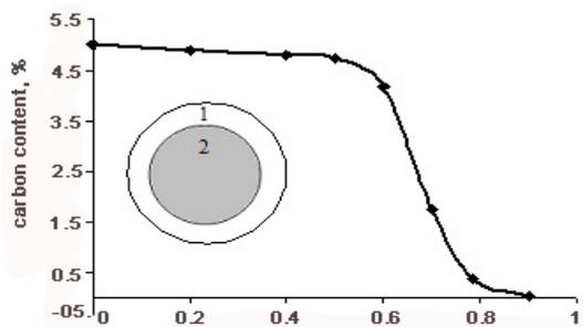
Fig. 5. Dependence of the carbon distribution in volume of the chromite pellets: 1 – a superficial light free-carbon layer; 2 – an internal dark carbon-containing layer.
