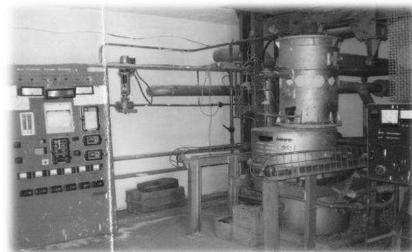
Fig. 3. A general view of the trial installation with a calcining bowl in volume of 0.3 m<sup>3</sup>.
