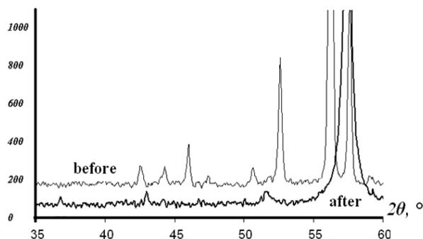
Fig. 4. XRD-pattern of the Sample 3 (before and after the heat treatment at 600 °C).
