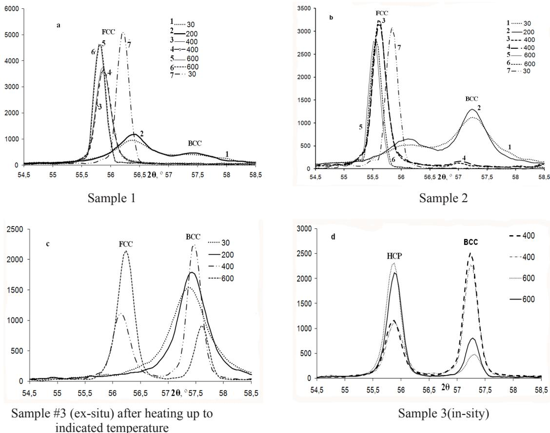
Fig. 3. XRD-patterns of the samples. Heating was performed in the following program 30-200-400-400 (keeping 1 h) -600-600 (keeping 1 h) – 30 °C.
