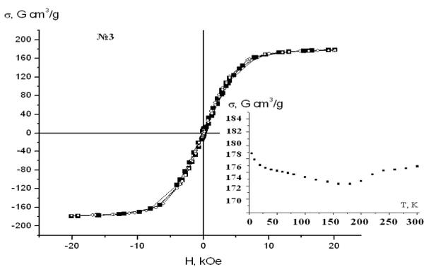
Sample 3, saturation magnetization and hysteresis parameters (remanence, coercivity)
