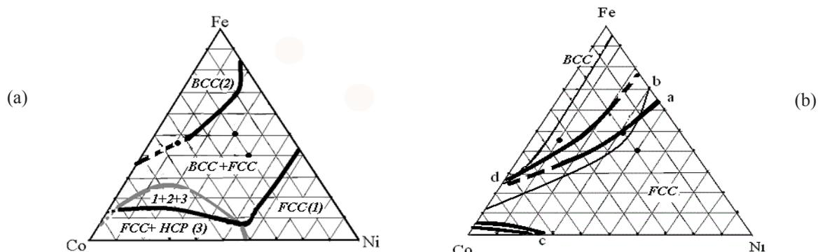
Fig. 1. Isothermal PDS of Fe-Co-Ni nanosystem at 30 °C (a) and at 500 and 600 °C (b) the system. The dots are discussed in the work.
