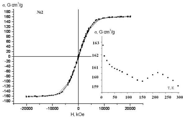
Sample 2, saturation magnetization and hysteresis parameters (remanence, coercivity)
