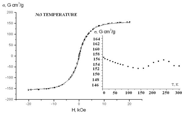
Sample 3, saturation magnetization and hysteresis parameters (residual magnetization, coercive force) after heat treatment
