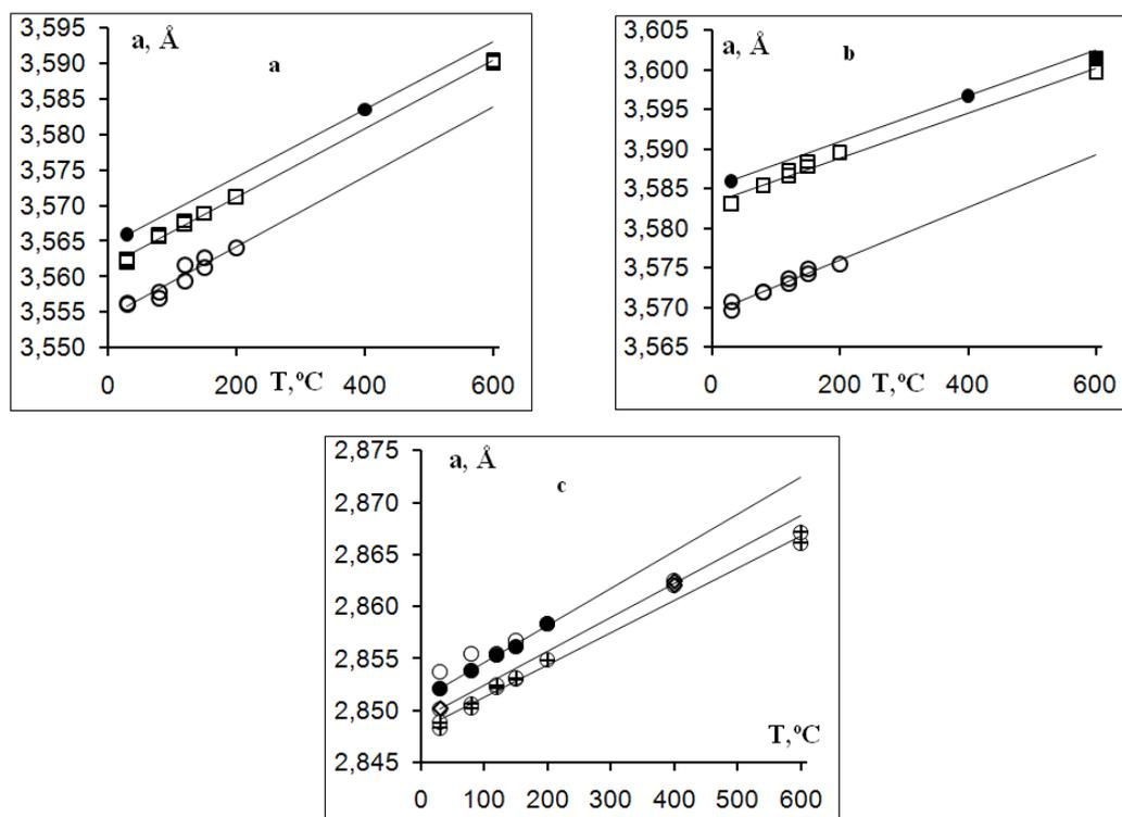
Fig. 5. The effect of temperature on the lattice parameter of cubic phases in the Samples #1 (a), # 2 (b), # 3 (c). Values of linear thermal expansion coefficients measured at heating up to 200, 400 and 600 °C, respectively: a)  $133 \cdot 10^{-5}$ ,  $136 \cdot 10^{-5}$ ,  $1.39 \cdot 10^{-5}$ ; b)  $8.06 \cdot 10^{-6}$ ,  $7.93 \cdot 10^{-6}$ ,  $9.33 \cdot 10^{-6}$ ; c)  $1.25 \cdot 10^{-5}$ ;  $1.15 \cdot 10^{-5}$  and  $1.09 \cdot 10^{-5}$ .
