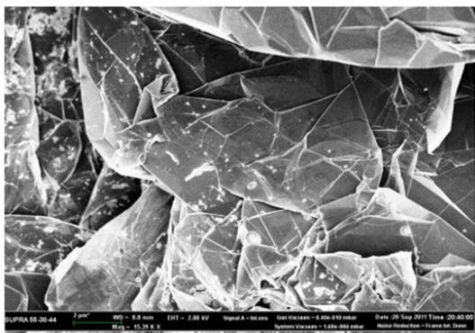
Fig. 3. Thermally expanded graphite surface decorated with Mg nanoparticles by MS.
