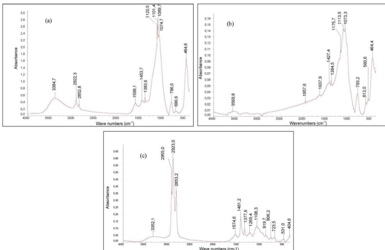
Fig. 9. FTIR spectra of TRH: (a) - TRH<sub>400</sub>; (b) - TRH<sub>700</sub> and (c) - TRH<sub>700</sub> after petroleum sorption.
