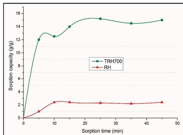
Fig. 2. Effect of contact time on sorption of heavy crude petroleum on TRH<sub>700</sub> and RH.
