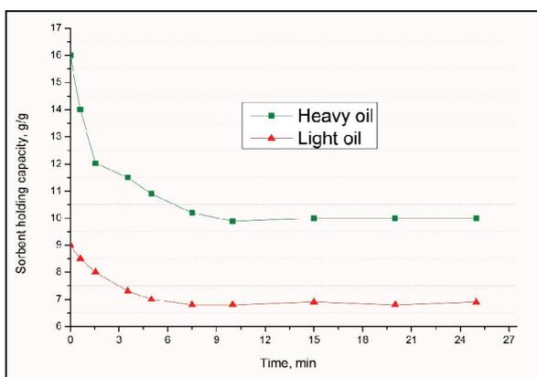
Fig. 4. Effect of desorption time on holding capacity of TRH<sub>700</sub>.
