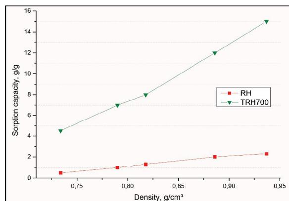
Fig. 3. Influence of adsorbate density on the sorption capacity for TRH<sub>700</sub> and RH.
