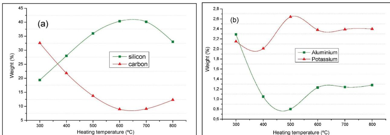
Fig. 6. Variation of weight percentage of silicon, carbon (a) and potassium, aluminum (b) in TRH produced at different temperatures.
