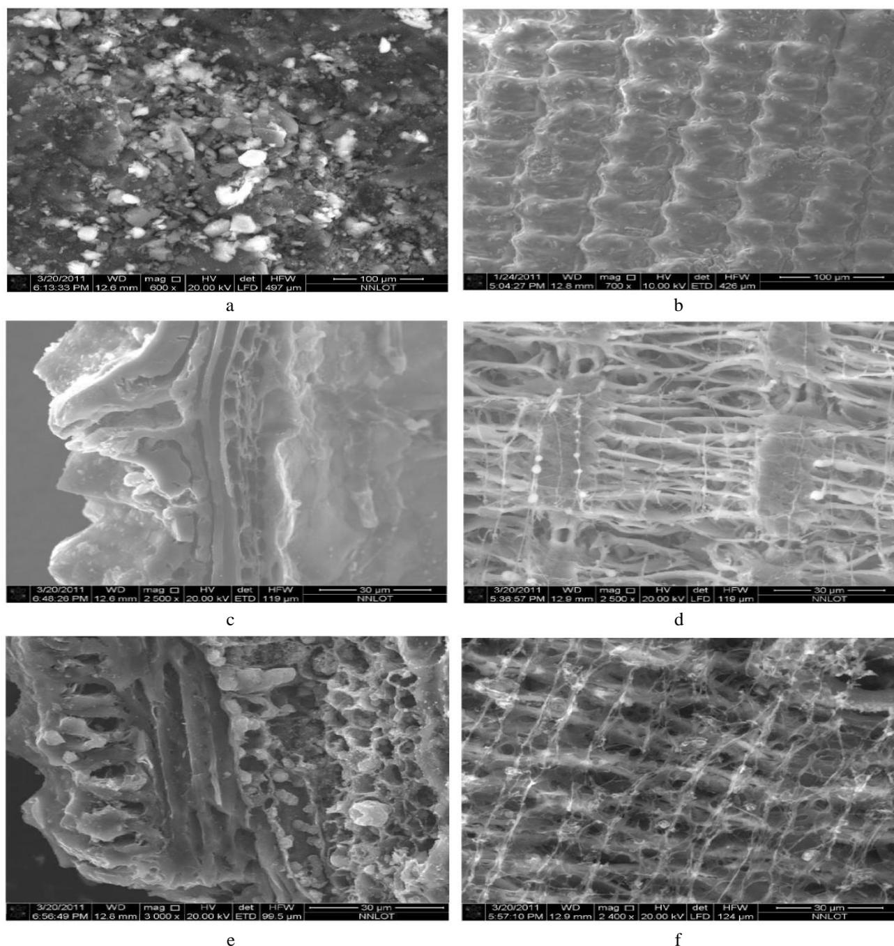
Fig. 10. SEM images of RH and TRH; (a)-RH, (b, c, d)-TRH<sub>400</sub> and (e, f)-TRH<sub>700</sub>.
