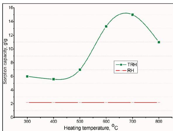
Fig. 1. Effect of heating temperature on heavy crude petroleum sorption properties of TRH<sub>700</sub> and RH.
