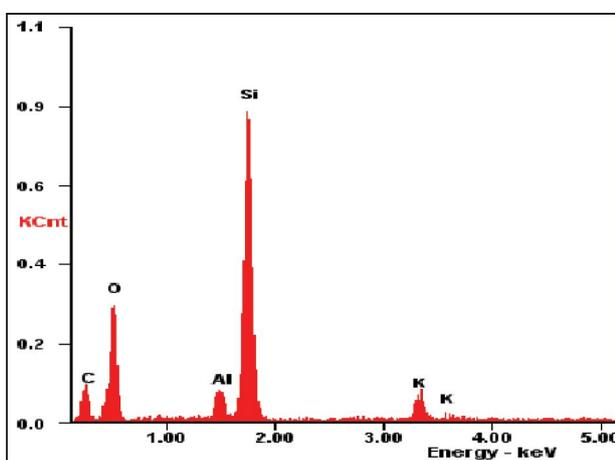
Fig. 7. Microanalysis of TRH<sub>700</sub> using SEM/EDAX.
