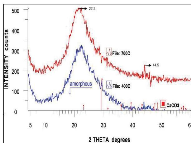
Fig. 8. XRD of the rice husk thermally treated at 400 °C and 700 °C.
