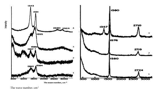
Fig. 10. Raman spectra according to [21] of noncrystalline (a), mostly graphite (b). (a) 1 – charcoal, 2- coke, 3 – diamond – like carbon, 4 – glassy carbon; (b) 1 – natural graphite, 2 – highly oriented pyrolytic graphite, 3 – polycrystalline graphite.
