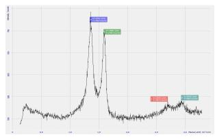
Fig. 7. Raman spectrum of schungite rock from "Bakyrchik" deposit.
