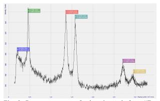
Fig. 8. Raman spectrum of schungite rock from "Zazhogino" deposit.
