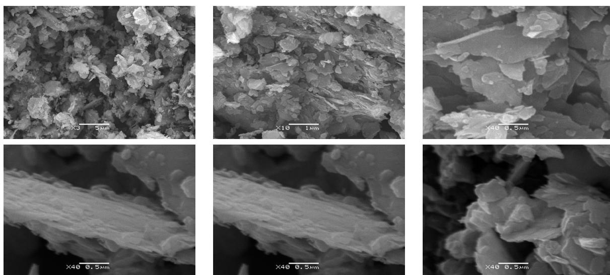
Fig. 5. Fragments of SEM images of carbon concentrate of schungite ore from "Bakyrchik" deposit at different magnification.
