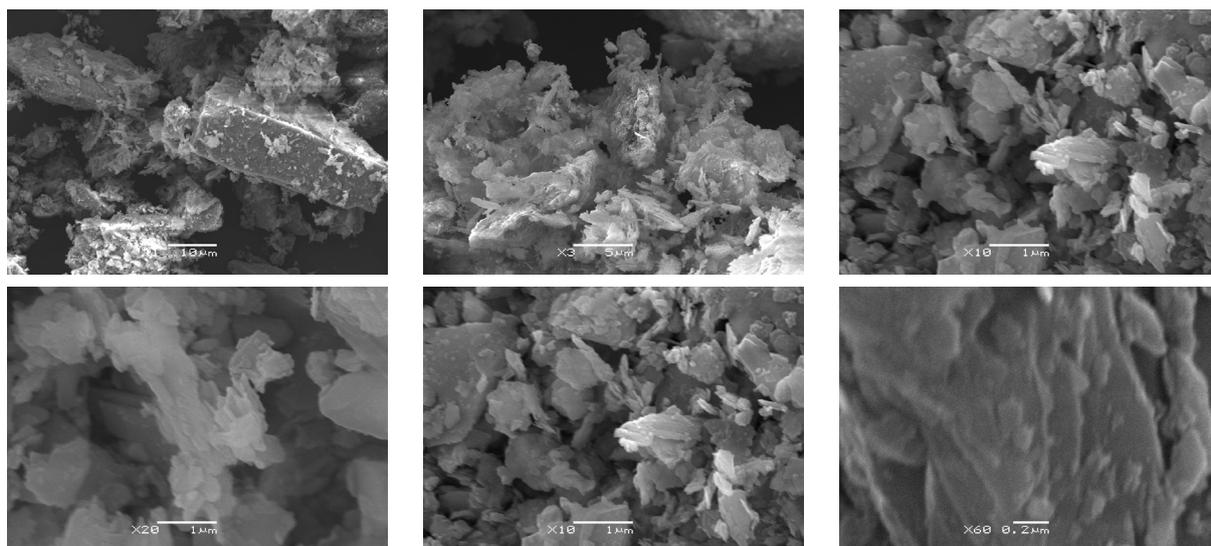
Fig. 4. Fragments of SEM images of schungite rock from "Bakyrchik" deposit at different magnification.
