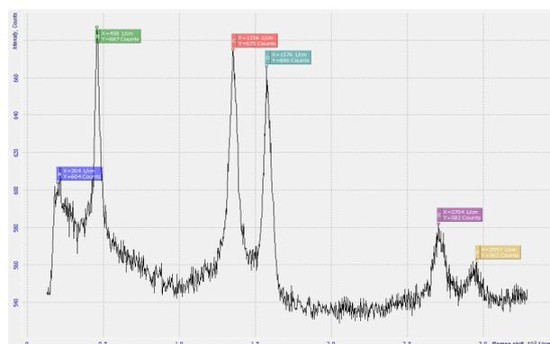
Fig. 9. Raman spectrum of shungite concentrates from "Bakyrchik" deposit.
