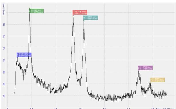
Fig. 8. Raman spectrum of shungite rock from "Zazhogino" deposit.
