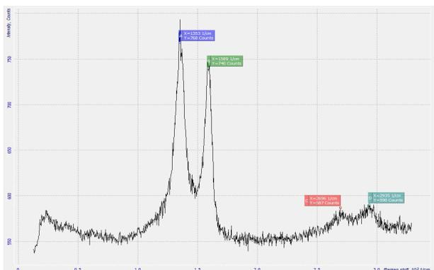
Fig. 7. Raman spectrum of shungite rock from "Bakyrchik" deposit.
