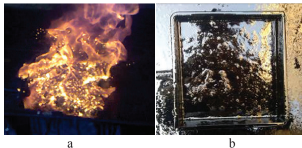
Fig. 3. The photo of an intensive combustion process with emission of vapor to the flame (a) and swelling process of oil mass after completion of burning due to continued boiling of water sub layer (b).
