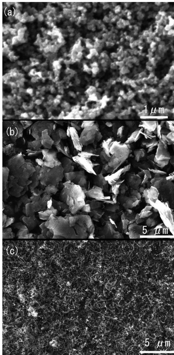
Fig. 1. SEM images of carbon black (a), graphite nanoparticles (b), and CSCNT (c).
