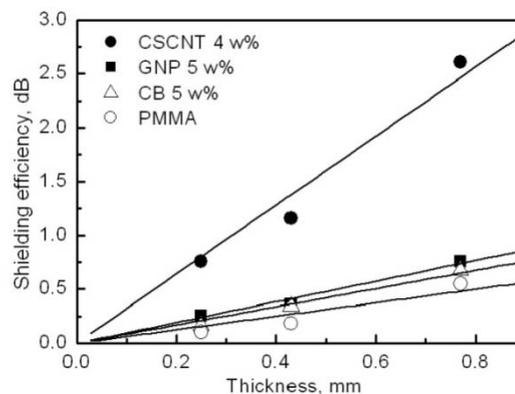
Fig. 5. Dependence of shielding efficiency on the sheets thickness.
