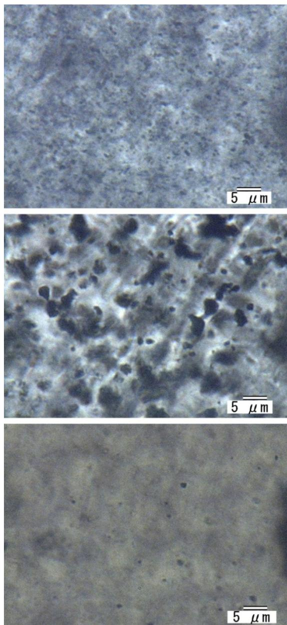
Fig. 2. Optical images of polymer sheets with dispersed carbon black, 1 w% (a), graphite nanoparticles, 1 w% (b), and CSCNT, 1 w% (c).
