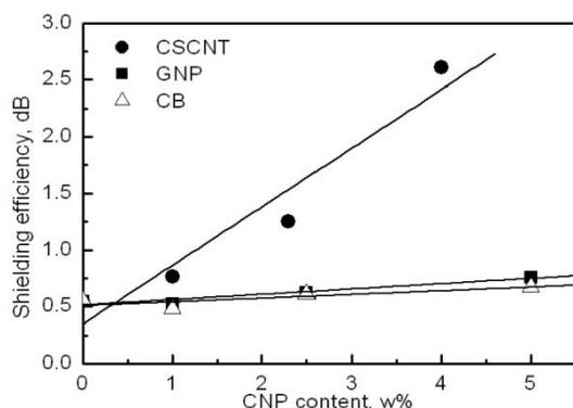
Fig. 4. Shielding efficiency of carbon nanoparticles (CNP) dispersed polymer composites as a function of CNP content.
