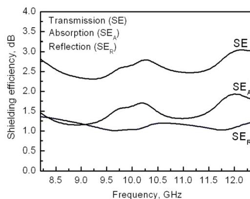
Fig. 3. Transmission, absorption and reflection of CSCNT(4 w%)/polymer composite (thickness 0.77 mm).
