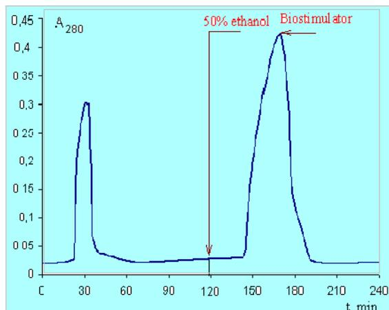
Fig. 1. The separation of biostimulator on nanocarbonsorb column
