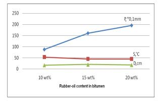
Fig. 5. Characteristics comparison of Rubber-bitumen compounds with not active rubber crumb (06-1)
