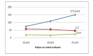
Fig. 4. Characteristics comparison of Rubber-bitumen compounds with active rubber crumb.
