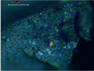
Fig. 1. Optical microscope images of rubber crumb with particle size less than 0.6 mm (active).
