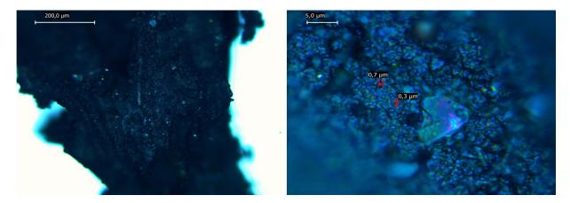
Fig. 2. Optical microscope images of rubber crumb with particle size 0.6-1.0 mm (non active).
