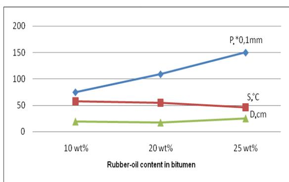
Fig. 4. Characteristics comparison of Rubber-bitumen compounds with active rubber crumb.
