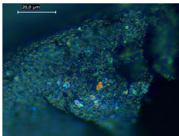
Fig. 1. Optical microscope images of rubber crumb with particle size less than 0.6 mm (active).
