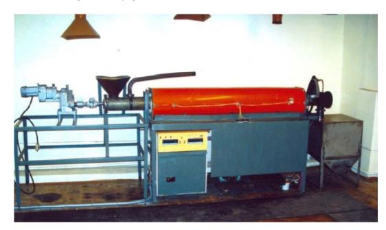
Fig. 1. Pilot setup for flame carbonization of diverse raw plant materials.
