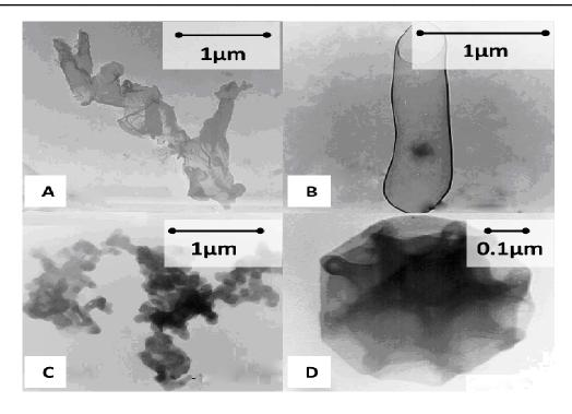
Fig. 3. Diverse micro- and nanoscale structures observed with electron microscopy in apricot stones carbonized at different temperatures: (A) at 500°C; (B) at 600°C for 30 min; (C) at 700°C; (D) at 750°C.
