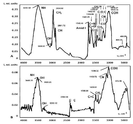
Fig. 5. IR-spectra of native (non-carbonized) (A) and carbonized at 800°C (B) apricot stone surfaces.
