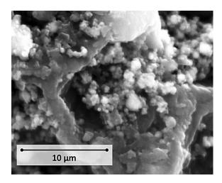
Fig. 13. Electron microphotograph of the heterogeneous bio-composite bioremediation material created on the basis of NCS and bacterial cells Pseudomonas aeruginosa.
