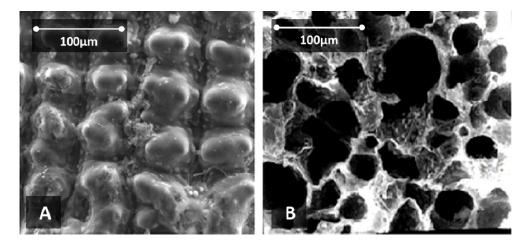
Fig. 2. Electron microscopic images of rice shells in native state (A) and after carbonization at 650°C (B).
