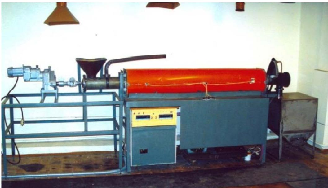
Fig. 1. Pilot setup for flame carbonization of diverse raw plant materials.
