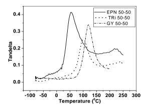
Fig. 5. DMA of different epoxy composites with 50/50 compositions-Variation of tan  $\delta$  with temperatures.
