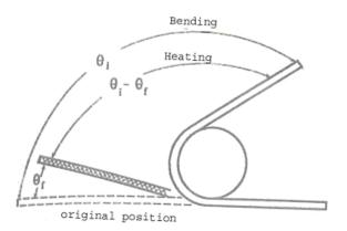
Fig. 1. Schematic representation of bending test.
