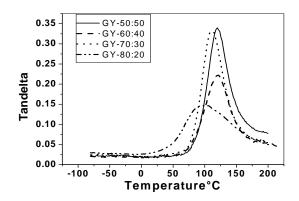
Fig. 3. Variation of tan  $\delta$  vs temperatures for GY/carbon composites.
