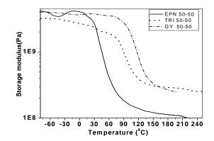
Fig. 4. DMA of different epoxy composites with 50/50 compositions; Variation of storage modulus with temperature.
