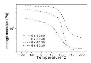
Fig. 2. Variation of storage modulus with temperature for the GY/ carbon composites.
