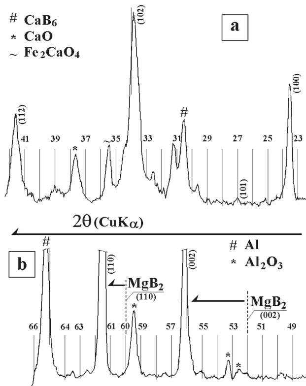
Fig. 3. X-ray data: a) system 2B-2C-Ca processed during 21 hours in mill  $\rightarrow$  2 after its annealing within 2 hours in a current atmosphere of argon at  $\sim 1000^\circ\text{C}$ , see PDF 34-952; 83-515; 82-1691; 74-2136; b) processing 2 hours, SPEX 8000 mill, the system 2B-0.5Mg-0.5Al, annealing time 2 hours, an atmosphere of argon,  $\sim 1000^\circ\text{C}$ , see PDF 8-263; 3-939; 12-539).
