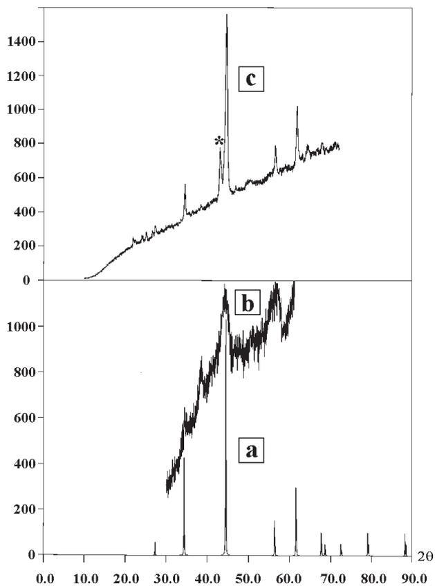
Fig. 1. X-ray data on the systems 2B-Al: a) standard  $\text{AlB}_2$  (see PDF No 39-1483); b) a product of mechanical activation within 90 minutes in the mill AGO-2; c) the same product after the thermal analysis in an atmosphere of argon up to  $900^\circ\text{C}$ ; the mark (\*) answers the most intensive reflex of compounds  $\text{Al}_x\text{Fe}_y$ , where the attitude  $x/y \geq 2.5$ .
