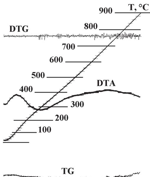
Fig. 2. Thermal analysis of mechanically activated system 2B-Al, processed during 90 min in mill AGO-2.
