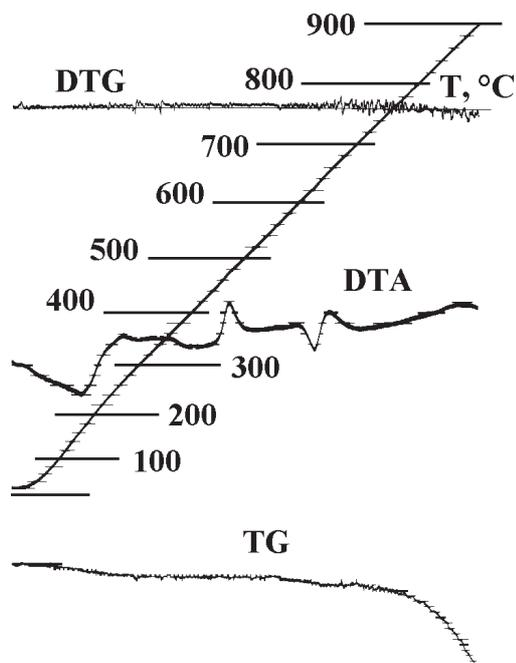
Fig. 4. Thermal analysis of mechanically activated system 2B-Mg, processed during 90 min in mill AGO-2.
