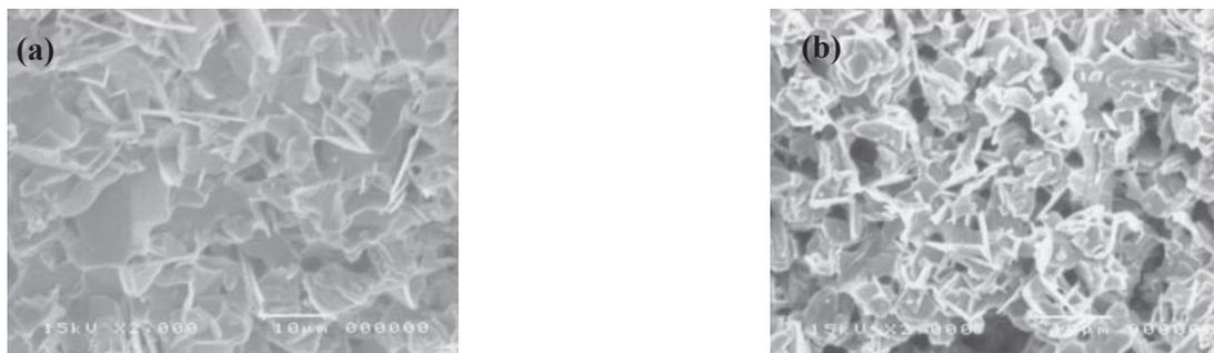
Fig. 5. SEM micrographs of samples deposited in butanol solvent; (a) heat-treated in vacuum and (b) in atmosphere.
