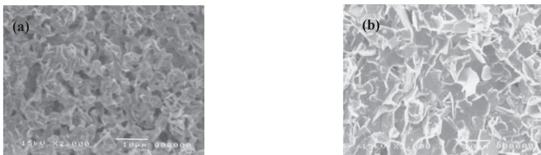
Fig. 6. SEM micrographs of samples deposited in Ethanol solvent; (a) heat-treated in vacuum and (b) in atmosphere.
