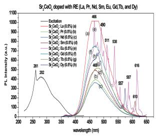
Fig.3. Excitation and emission of RE<sup>3+</sup> (0.5%) doped Sr<sub>2</sub>CeO<sub>4</sub> phosphor
