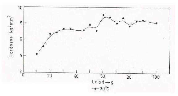
Fig. 2. Vickers indentation impure carbazole
