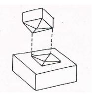
Details of the diamond pyramid indenter together with its impression
