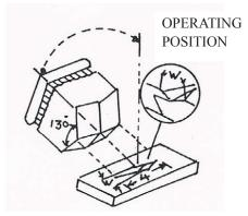
Details of the knoop indenter together with its impression
