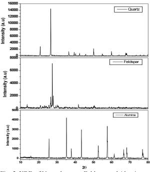
Fig. 5. XRD of Natural quartz, Feldspar and Alumina.
