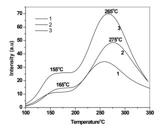
Fig. 3. Curves 1,2, and 3 are the TL of 200, 400 and 800AQ of alumina ( $Al_2O_3$ ).
