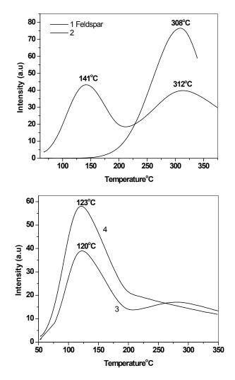
Fig. 2. Curves 1,2, 3 and 4 are the NTL, 200, 400 and 800AQ of Feldspar.
