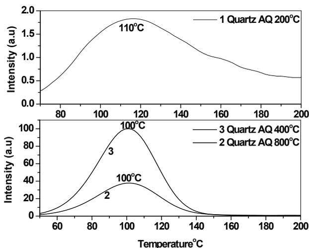
Fig.1. Curve 1 is the TL of 15Gy beta dose natural quartz annealed and quenched form 200°C.
