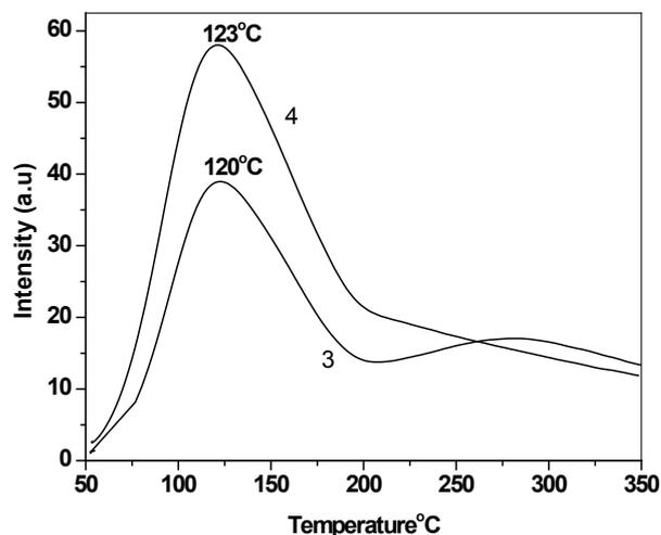
Fig. 2. Curves 1,2, 3 and 4 are the NTL, 200, 400 and 800AQ of Feldspar.
