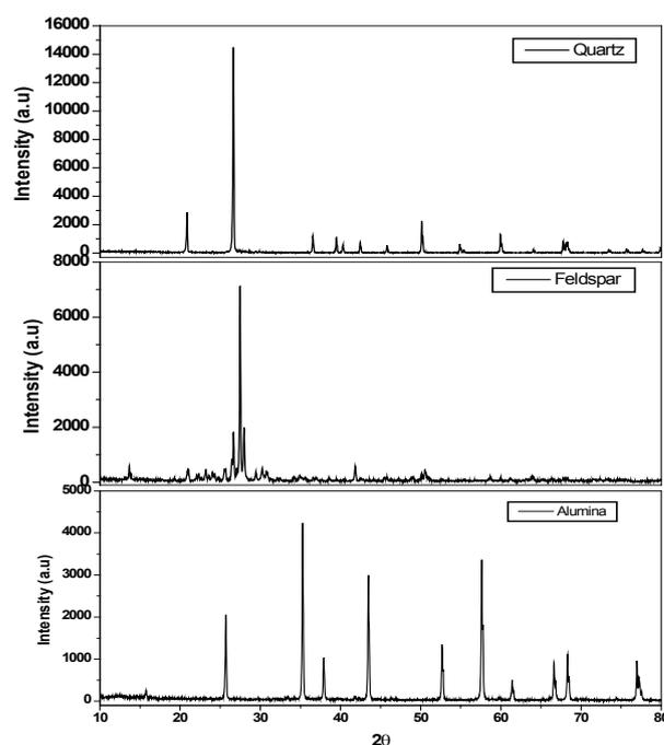
Fig. 5. XRD of Natural quartz, Feldspar and Alumina.
