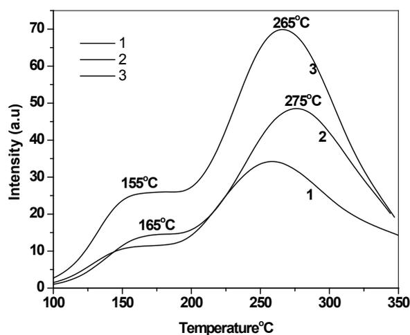
Fig. 3. Curves 1,2, and 3 are the TL of 200, 400 and 800AQ of alumina ( $\text{Al}_2\text{O}_3$ ).
