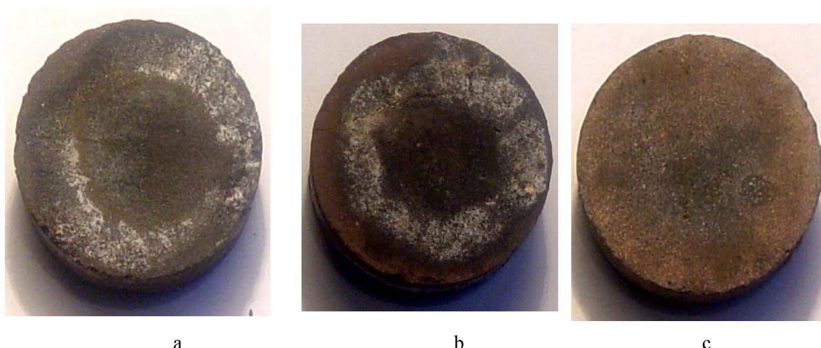
Fig. 12. External view of samples, synthesized on the base of non-active (a), activated (b) and modified (c) quartz
