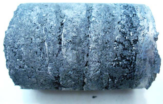
Fig. 7. The macrostructure of the combustion product in the system (NiO + Al + \text{Al}_2\text{O}_3 ) proceeding in the mode of self-sustained oscillations under the effect of centrifugal acceleration
