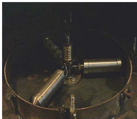
Fig. 2. The main unit of the centrifuge for investigation of furnace-out combustion processes under the effect of centrifugal forces
