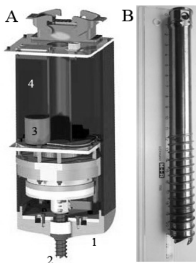
Fig. 1. (A) The melting probe IceMole has been developed at Aachen University of Applied Sciences, Aerospace Technology Department. The probe consists of the copper melting head (1), containing four heaters, which it can melt through the thick ice sheet. To ensure the advancement of the probe in the dirty ice, an ice screw (2) driven by a small motor (3) is attached, which can facilitate drilling through layers of non-melting material. The measurement equipment can be loaded into the rear chamber of the device (4) made of aluminium. (B) The stainless steel screw used in this microbiological study is shown together with a 20 cm-long scale.
