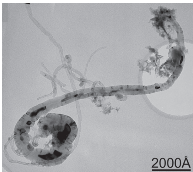
Fig. 7. Micrograph of the filamentary carbon formed from methane on the 85%Ni/Al 2 O 3 catalyst at 750°C.
