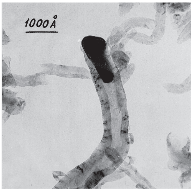
Fig. 9. Micrograph of the filamentary carbon formed from methane diluted with hydrogen ( \text{CH}_4:\text{H}_2 = 1:1 ) on the 85% Ni/ \text{Al}_2\text{O}_3 catalyst at 700°C.
