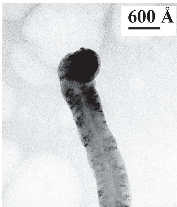
Fig. 4. Micrograph of the filamentary carbon formed from methane on the 85%Ni/Al 2 O 3 catalyst at 550°C (the carbon concentration in the sample is 900 wt.% relative to the catalyst weight).
