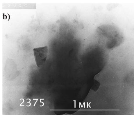
Fig. 2. A roentgenogram (a) of starting quartz (I) and dispersed in planetary-centrifugal mill (II). Electron-microscopic image (b) of quartz particle abraded in mill.
