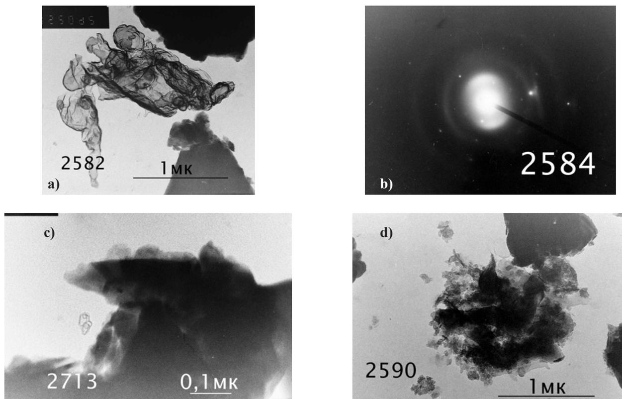
Fig. 4. Quartz electron-microscopic images (a, c, d) and electronogram (b) dispersed in planetary-centrifugal mill with 5% polysterene.
