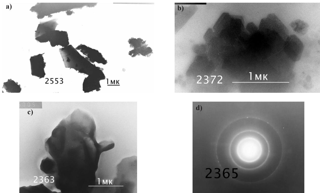
Fig. 1. Quartz electron-microscopic images after dry abrading in agate vessel (a) and in the presence of alcohol (b, c); a picture of carbonic substance diffraction on the quartz specimen abraded in alcohol (d) (1 mk = 1  $\mu\text{k}$ ).
