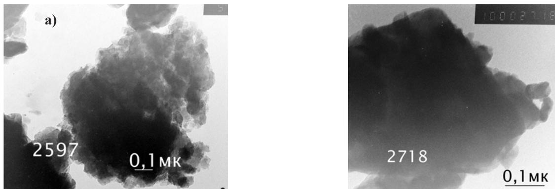
Fig. 5. Quartz electron-microscopic images dispersed in planetary-centrifugal mill with 5 % carbon.
