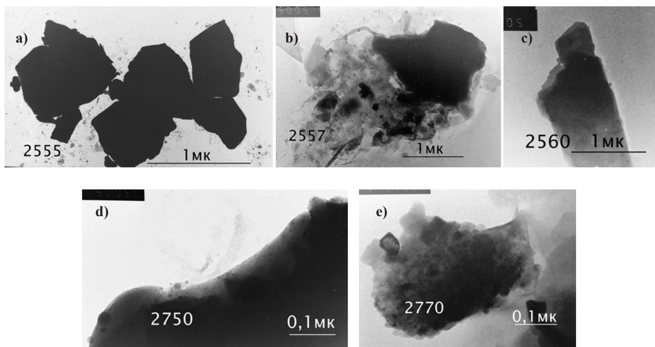
Fig. 3. Electron-microscopic pictures of quartz powder particles dispersed in planetary-centrifugal mill with butyl alcohol.
