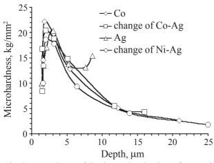
Fig. 3. Dependence of depth on microhardness for metallized Kapton 100 HN films.
