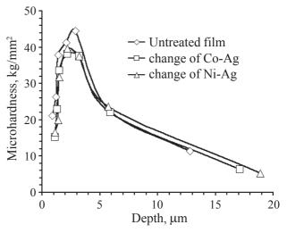
Fig. 4. Dependence of depth on microhardness for metallized Upilex 25F films.
