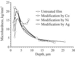
Fig. 2. Dependence of depth on microhardness for metallized Kapton 100 HN films.
