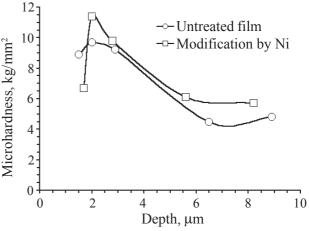
Fig. 1. Dependence of depth on microhardness for metallized Kapton 50 HN films.
