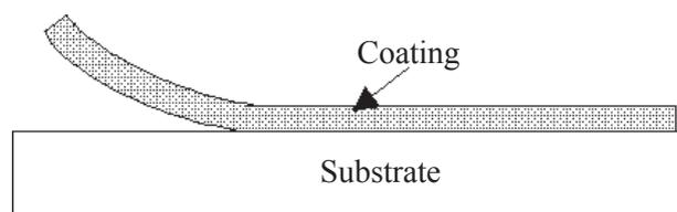
Fig. 6. Schematic drawing of a coating debonding from a substrate.
