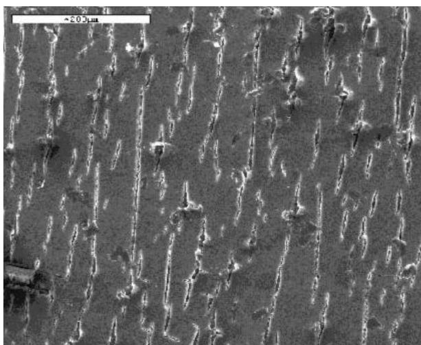
Fig. 4. SEM image of cracks in an Ag-Ni metallized coating of a 75 micron-thick Kapton after tensile failure.
