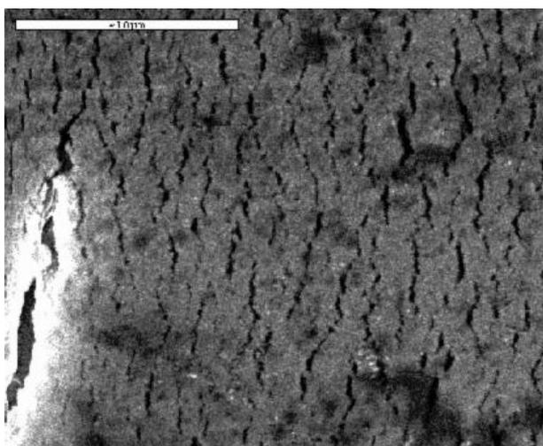
Fig. 5. Higher magnification SEM image of cracks in an Ag-Ni metallized 75 micron-thick Kapton.
