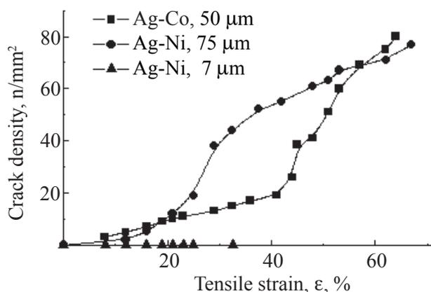
Fig. 3. Linear density of the cracks plotted against tensile strain.
