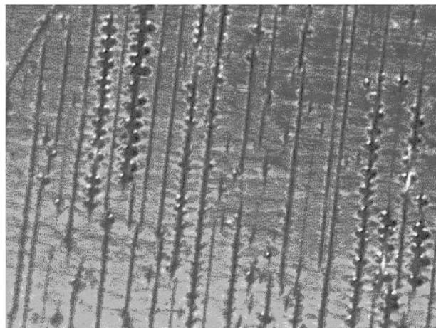
Fig. 2. An optical micrograph of Ag-Co metallized surface of a 50 micron-thick Kapton substrate after tensile failure.
