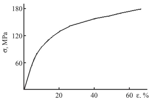
Fig. 1. Typical stress-strain curve for a metallized Ag-Co/Kapton film. The film thickness is 50 microns.
