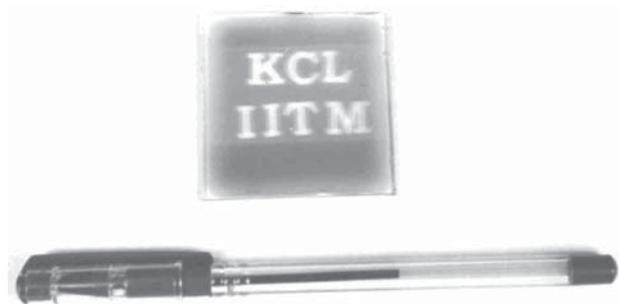
Fig. 6. Photograph of PVA-SiO<sub>2</sub>-PW composite coated on glass plate and irradiate under sunlight for 15 min.
