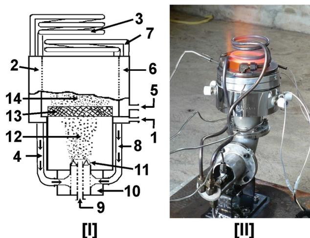
Fig. 9. Schematic illustration [I] and experimental view [II] relating with the self-circulation combustion process aided with waste-heat: 1 – solution circulation with excess-heat; 2 – fuel circulation with excess-heat; 3 – evaporation tube of solution; 4 – fuel evaporation tube; 5 – steam pipe; 6 – high-temperature fuel pipe; 7 – flow mixer; 8 – spray nozzles; 9 – solution inlet; 10 – fuel inlet; 11 – air inlet; 12 – baffle plate (Cu-mesh); 13 – mixing space; 14 – burning space.
