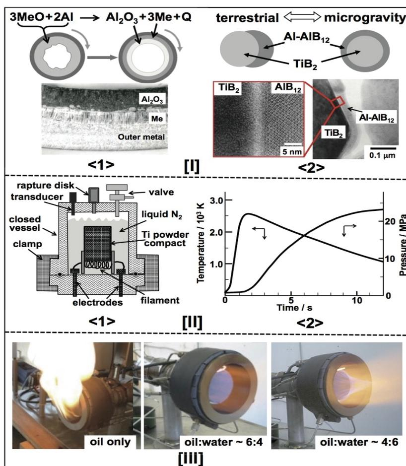
Fig. 2. Typical performances with the aids of inertia-forces and excess-heat. [I] Gravitational composite formations under high-g <1> and  $\mu$ -g <2>. [II] TiN combustion synthesis with liquid N<sub>2</sub>; <1> closed-type apparatus, <2> T and P changes during the process. [III] Self-circulation with activated waste-heat.
