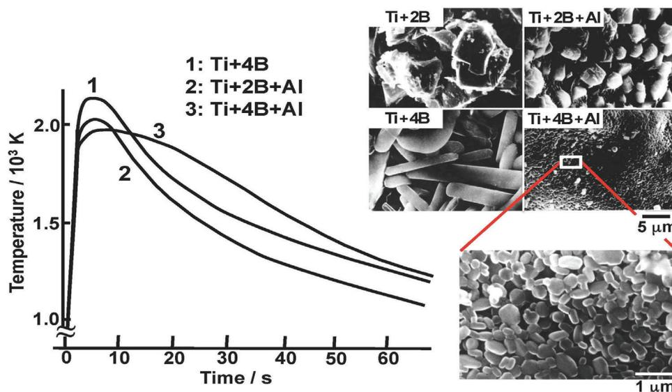
Fig. 4. Typical results obtained on Ti-B-Al system for  $\text{TiB}_2\text{-AlB}_{12}\text{-Al}$  nano-composite particle synthesis.
