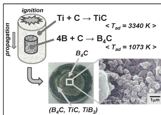
Fig. 6. Typical results obtained in the R&D on B-C system for  $\text{B}_4\text{C}$  formation with the aid of Ti-C combustion synthesis as a chemical oven.
