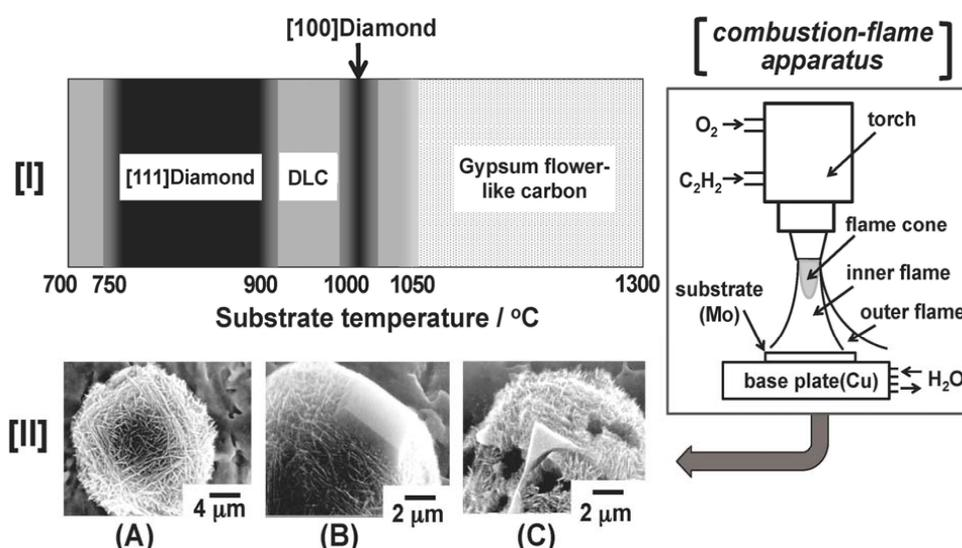
Fig. 5. Typical results obtained in the R&Ds on C-allotropes formed with a combustion-flame method. [I]: Temperature ranges for carbon allotropes formation; [II]: Changes from gypsum flower-like carbon to diamond.
