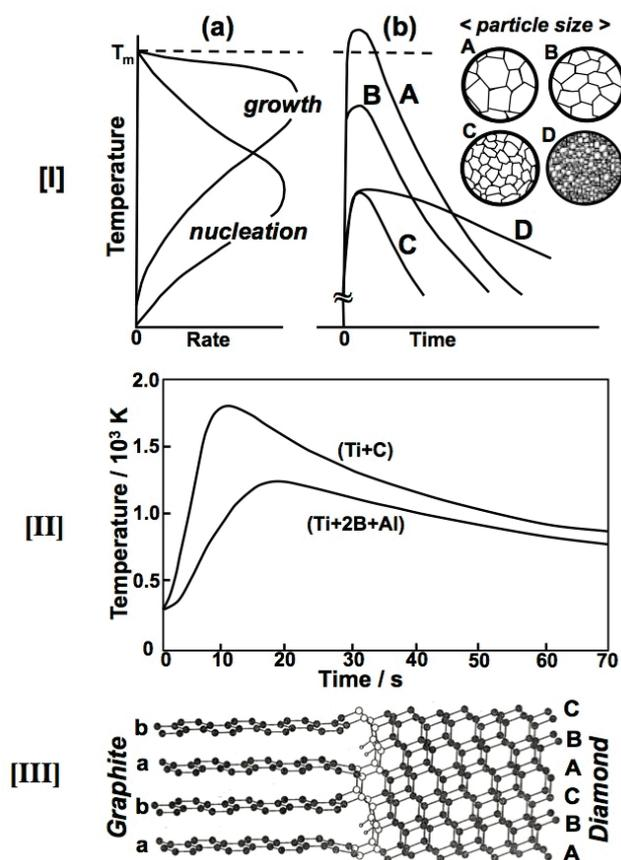
Fig. 3. Precursors supplies followed by nano- and low-density compounds synthesis. [I] high-temperature gradients; Ti-B-Al systems, Sr-Al-O systems. [II] chemical oven and waste-heat utilization; B-C systems, Ti-N systems. [III] phase transformation design from graphitic prism to diamond nucleation.
