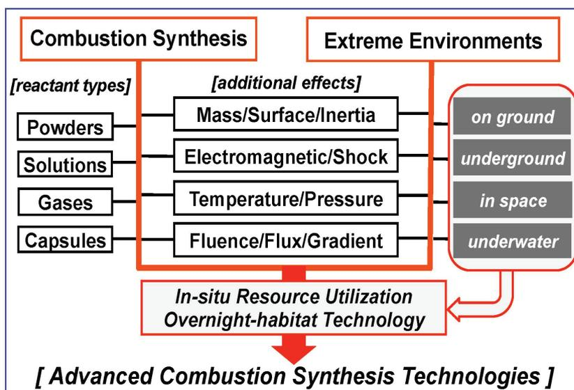
Fig. 1. Schematic design systematically categorized in extreme environments with additional effects and varieties of reactant selections.
