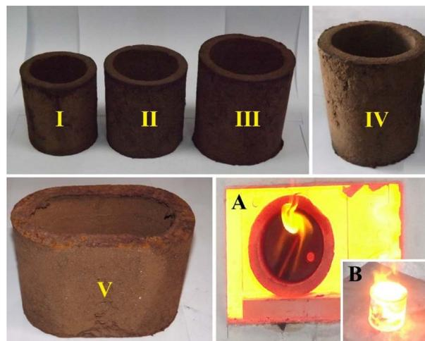
Fig. 2. Photographs of exothermic riser sleeves before performance tests and during tests; (A) riser sleeve in the muffle furnace, (B) riser sleeve during cooling period.
