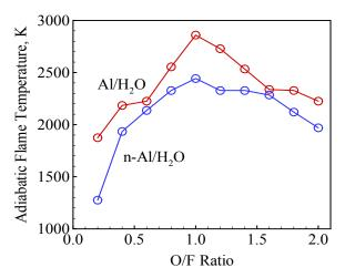
Fig. 1. Effect of oxidizer-fuel weight (O/F) ratio on the adiabatic flame temperature of  $Al/H_2O$  mixtures; oxide content in nanoparticles is 50% by mass.
