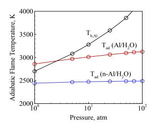
Fig. 2. Effect of pressure on the adiabatic flame temperature of stoichiometric Al/H<sub>2</sub>O mixtures; oxide content in nanoparticles is 50% by mass.
