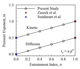
Fig. 10. Pressure exponent as a function of entrainment index for diffusion and kinetic controlled combustion mechanisms (reprinted from [22] with permission of Elsevier).
