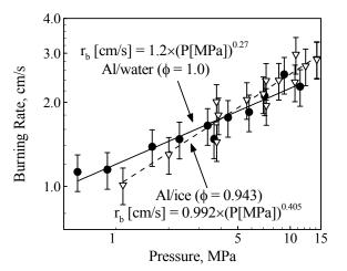
Fig. 6. Effect of pressure on the burning rate of 80 nm  $Al/H_2O$  mixture (reprinted from [14] with permission of American Institute of Aeronautics and Astronautics).
