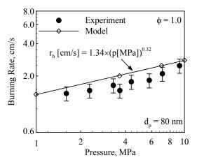
Fig. 8. Effect of pressure on burning rate of stoichiometric Al-H<sub>2</sub>O mixtures containing 80 nm particles (reprinted from [5] with permission of Elsevier).
