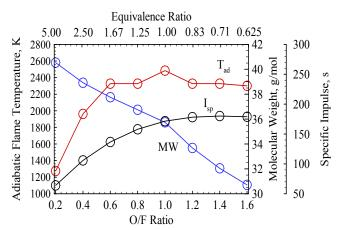
Fig. 3. Sea-level specific impulse, adiabatic flame temperature, and product molecular weight of Al- $H_2O$  propellant as a function of O/F ratio; theoretical calculations for a chamber pressure of 50 atm and product expanded to atmospheric pressure.
