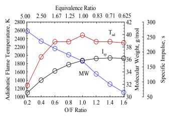
Fig. 4. Sea-level specific impulse, adiabatic flame temperature, and product molecular weight of n-Al- $H_2O$  propellant as a function of O/F ratio; theoretical calculations for a chamber pressure of 50 atm, particle oxide content of 50 wt.%, product expanded to atmospheric pressure.
