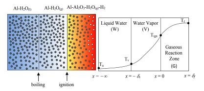
Fig. 7. Physical model and multi-zone flame structure (• Al,  $\circ$  Al<sub>2</sub>O<sub>3</sub>) (reprinted from [5] with permission of Elsevier).
