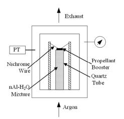
Fig. 5. Schematic of the constant-pressure strand burner with optical access (reprinted from [5] with permission of Elsevier).
