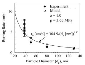
Fig. 9. Effect of particle size on burning rate of stoichiometric Al-H<sub>2</sub>O mixture at 3.65 MPa (reprinted from [5] with permission of Elsevier).
