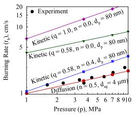
Fig. 11. Effect of pressure on the burning rate of stoichiometric aluminum-water mixture containing 80 nm particles (reprinted from [22] with permission of Elsevier).
