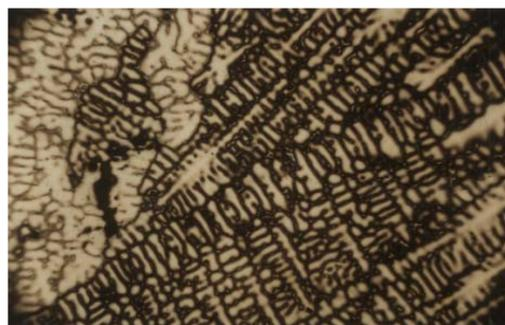
Fig. 4. Microstructure of Al-Si-Fe-Cu alloy system ( $\times 200$ ).
