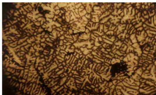
Fig. 10. Microstructure of Al-Si-Fe-Cu Alloy (0.3% Mn) ( $\times 200$ ).
