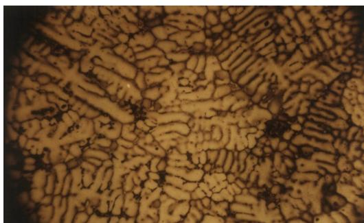
Fig. 6. Microstructure of Al-Si-Fe-Cu Alloy containing 0.2% Cr ( $\times 200$ ).
