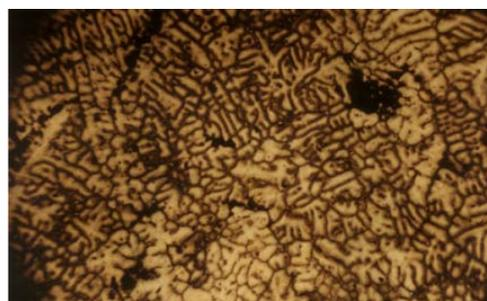
Fig. 11. Microstructure of Al-Si-Fe-Cu Alloy (0.1% Cr - 0.1% Mn) ( $\times 200$ ).
