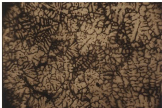
Fig. 13. Microstructure of Al-Si-Fe-Cu Alloy (0.3% Cr - 0.3% Mn) ( $\times 200$ ).
