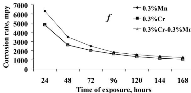
Fig. 1. Variation of corrosion rate with time of exposure for various additions: *a* – for chromium addition; *b* – for manganese addition; *c* – for combine addition of manganese and chromium; *d* – at 0.1% addition of chromium and manganese; *e* – at 0.2% addition of chromium and manganese; *f* – at 0.3% addition of chromium and manganese.
