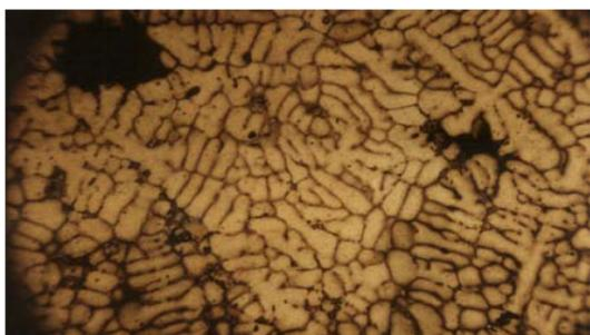
Fig. 7. Microstructure of Al-Si-Fe-Cu Alloy containing 0.3% Cr ( $\times 200$ ).
