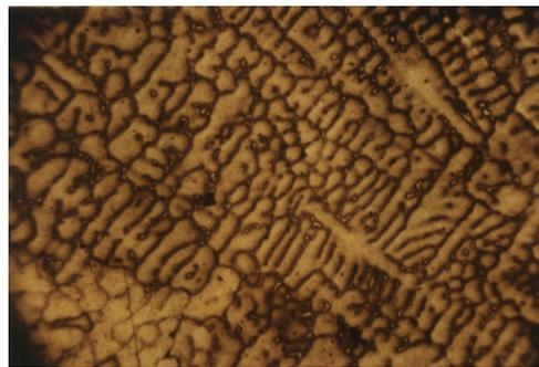
Fig. 9. Microstructure of Al-Si-Fe-Cu Alloy (0.2% Mn) ( $\times 200$ ).
