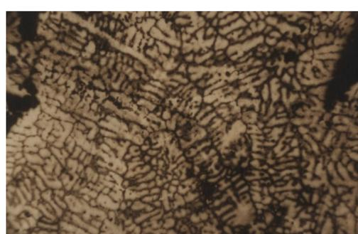
Fig. 12. Microstructure of Al-Si-Fe-Cu Alloy (0.2% Cr - 0.2% Mn) ( $\times 200$ ).
