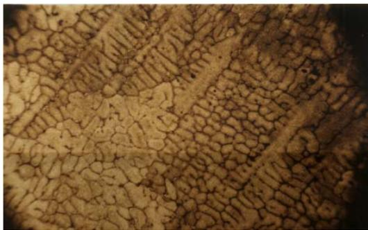
Fig. 5. Microstructure of Al-Si-Fe-Cu Alloy containing 0.1% Cr ( $\times 200$ ).
