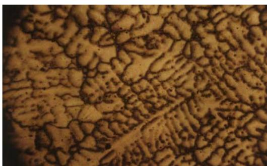
Fig. 8. Microstructure of Al-Si-Fe-Cu Alloy containing 0.1% Mn ( $\times 200$ ).
