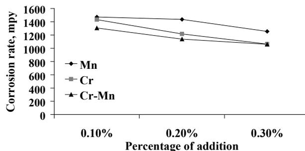
Fig. 3. Variation of corrosion rate with percentage addition of chromium and manganese at 168 hours.
