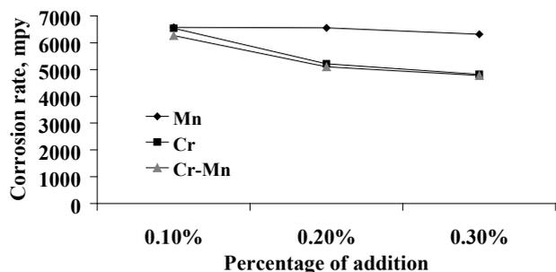
Fig. 2. Variation of corrosion rate with percentage addition of chromium and manganese at 24 hours
