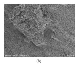
Fig. 4. SEM images of AS-FWCNT electrode: (a) – 100 times magnification; (b) –10000 times magnification.
