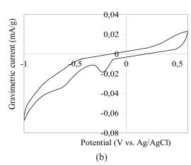
Fig. 2. (a) Specific capacitance and (b) CVs of FWCNT electrodes.
