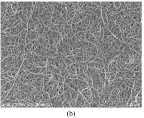
Fig. 1. SEM images of FWCNT papers: (a) – magnification of 30 000 times; (b) – magnification of 100 000 times.
