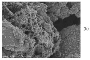
Fig. 5. SEM images of WS-FWCNT electrodes: (a) -300 times magnification; (b) -10000 times magnification.
