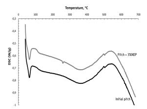
Fig. 7. DSC curves of initial pitch and pitch modified by NDP.
