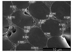
Fig. 11. Scheme of determination of surface area of the gap between fiber and matrix (values are given in square  $\mu$ m).
