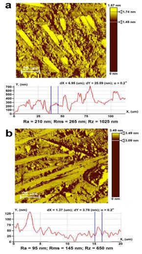
Fig. 12. Friction surface contour plot of CC0 (a) and CC3 (b) composites.
