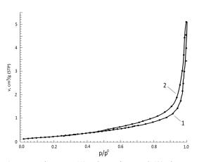
Fig. 6. 77 K nitrogen (1) adsorption and (2) desorption isotherms of C/C composites.
