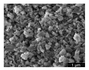
Fig. 1. SEM microphotograph of nanodiamond powder.
