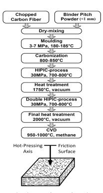
Fig. 2. General scheme of manufacturing process for C/C composites under study.
