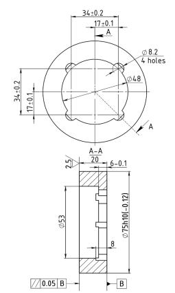
Fig. 4. Drawing of studied ring (stator and rotor).
