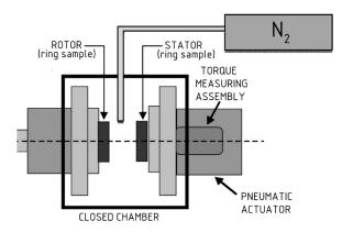
Fig. 3. Schematic diagram of subscale ring-on-ring.
