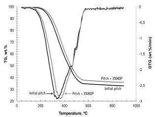
Fig. 8. TG and DTG curves of initial pitch and pitch modified by NDP.
