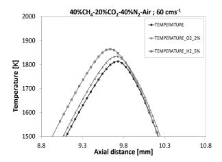
Fig. 4. Numerical solutions for temperature change in 40%  $CH_4 - 40\%$   $CO_2 - 20\%$   $N_2 -$  air (case A) flames with an addition of 2%  $O_2$  or 5%  $H_2$  at 60 cm s<sup>-1</sup> (left) and 40%  $CH_4 - 20\%$   $CO_2 - 40\%$   $N_2 -$  air (case B) flames with an addition of 2%  $O_2$  or 5%  $H_2$  at 60 cm s<sup>-1</sup> (right).
