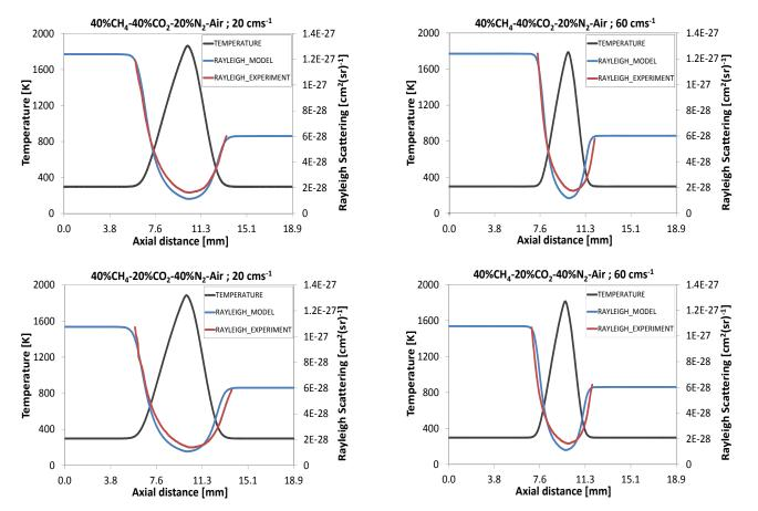
Fig. 3. Experimental and numerical solutions for 40%  $CH_4 - 40\%$   $CO_2 - 20\%$   $N_2$  – air (case A) at 20 cm s<sup>-1</sup> (top left) and 60 cm s<sup>-1</sup> (top right); 40%  $CH_4$  –20%  $CO_2$  – 40%  $N_2$  – air (case B) at 20 cm s<sup>-1</sup> (bottom left) and 60 cm s<sup>-1</sup> (bottom right).
