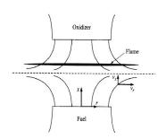
Fig. 2. Schematic of the experimental set-up (left) and counter flow flame (right) [15].
