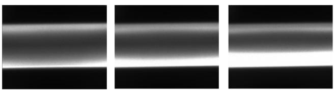
Fig. 1. Rayleigh signal (corresponding to temperature fields for diluted non-premixed  $CH_4 - N_2 - CO_2$  – air flames (top: air side; bottom: fuel side); at velocities of 20 cm s<sup>-1</sup>, 40 cm s<sup>-1</sup> and 60 cm s<sup>-1</sup> (left to right).
