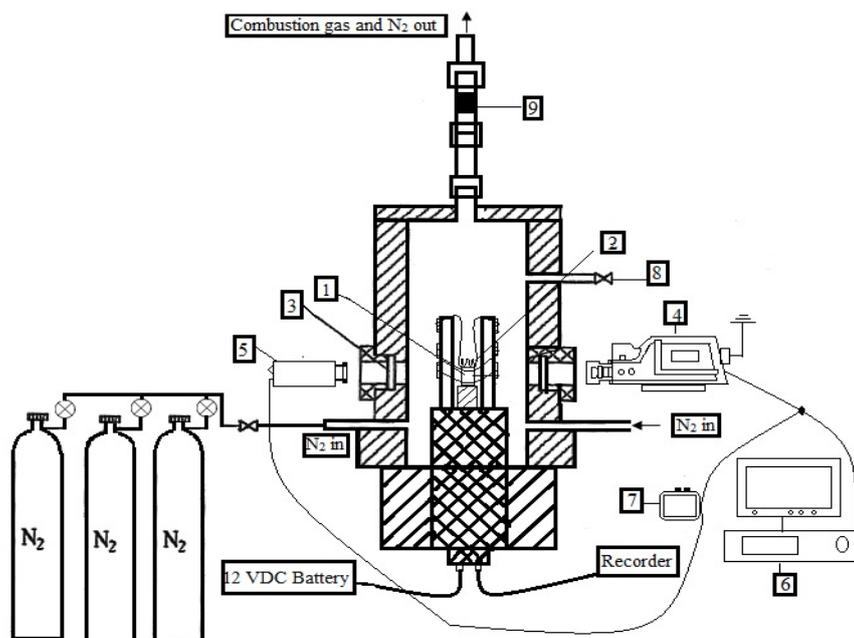
Fig. 1. Scheme of the combustion chamber under pressure: 1 – sample; 2 – nichrome wire; 3 – window; 4 – high-speed video camera; 5 – camera; 6 – transformer; 7 – PC; 8 – system for pressure control; 9 – filter.
