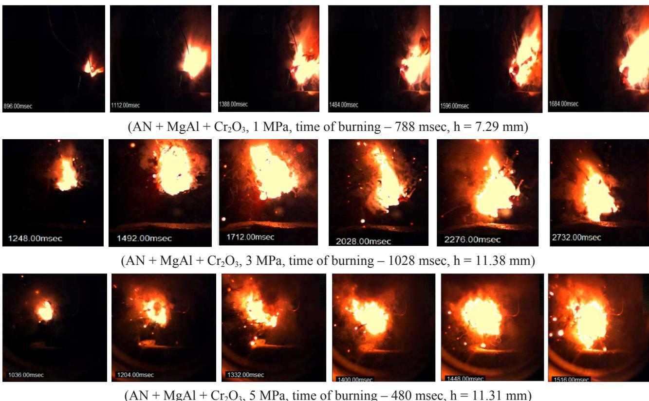
Fig. 3. Cinegrams of combustion of gas generator based on AN/MgAl/Cr<sub>2</sub>O<sub>3</sub> at 1 MPa, 3 MPa and 5 MPa.
