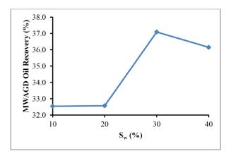
Fig. 2. Oil recovery under MWAGD for different initial water saturation in porous media.
