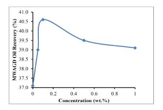
Fig. 3. Average oil recovery under MWAGD under microwave heating for  $Al_2O_3$  nanoparticles.
