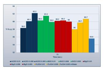
Fig. 1. Temperature alteration of deionized water and different water/nanofluid mixtures under microwave radiation
