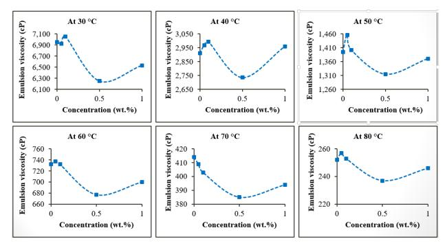
Fig. 4. Effect of nanofluid on emulsion viscosity.
