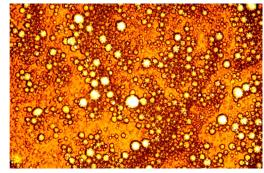
Fig. 5. Microphotograph of model water-oil emulsion (temperature -20 °C, water cut of the emulsion -30% by volume, dispersing time -3 min, the speed of the agitator of the disperser is -1500 rpm).
