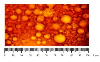
Fig. 1. Micrograph of a natural water-oil emulsion.
