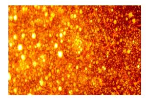
Fig. 2. Photomicrograph of the "old" of field water-oil emulsion during 1.5 months.
