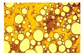
Fig. 4. Microphotograph of model water-oil emulsion (temperature -20 °C, water cut of the emulsion -40%, dispersion time -1 min, number of revolutions of the stirring device (mixer) of the disperser -1000 rpm).
