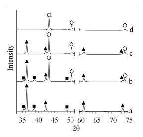
Fig. 1. X-ray phase analysis diagram of EG sample prepared with addition  $10\% \text{ Cu}(\text{NO}_3)_2$ . The samples were heat treated at: (a) 800 °C in air; (b) 1000 °C in air; (c) 1200 °C in air; (d) 1200 °C in nitrogen. The peaks have been assigned to Cu ( $\circ$ ), Cu<sub>2</sub>O ( $\blacktriangle$ ), CuO ( $\blacksquare$ ).
