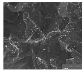
Fig. 2. SEM images of exfoliated graphite sample prepared with addition 10% Cu(NO<sub>3</sub>)<sub>2</sub>.
