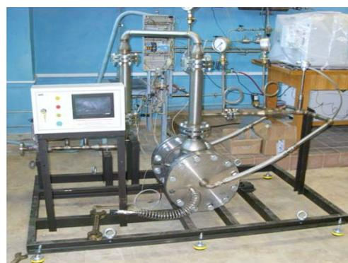
Fig. 5. Different types of pilot matrix converters with gas flows up to 10 m<sup>3</sup>/h.
